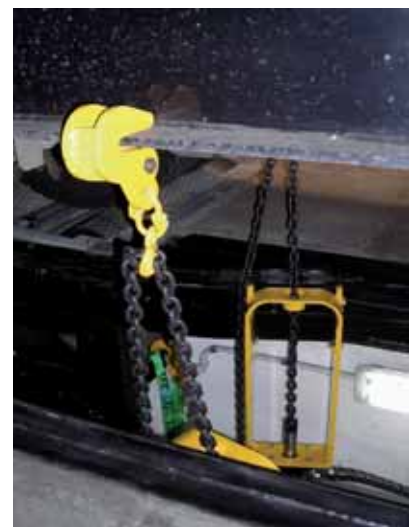
Load Simulation by chassis tie down. Picture kindly supplied by VTNZ.
