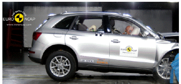
Offset crash test at 64km/h
