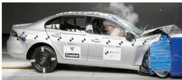
Offset crash test at 64km/h
