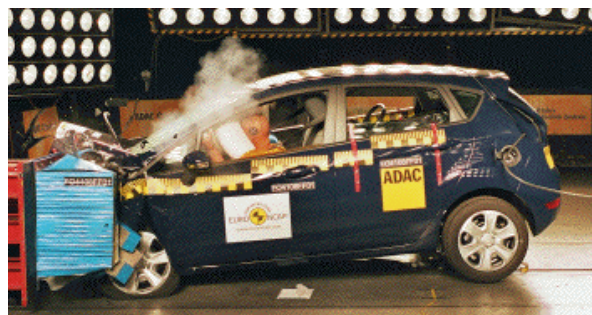
Offset crash test at 64km/h
