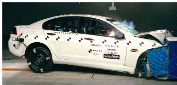
Offset crash test at 64km/h
