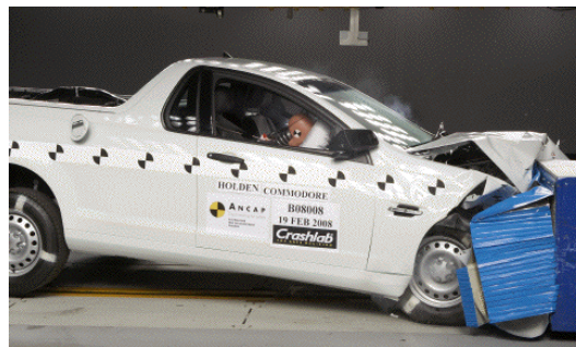
Offset crash test at 64km/h
