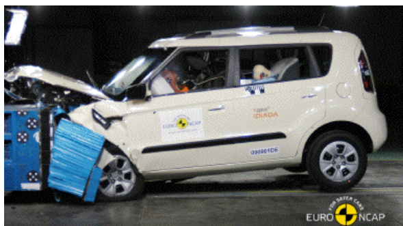
Offset crash test at 64km/h
