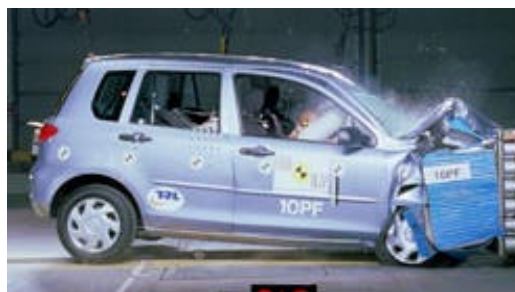
Offset crash test at 64km/h
