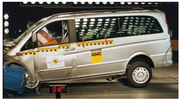
Offset crash test at 64km/h
