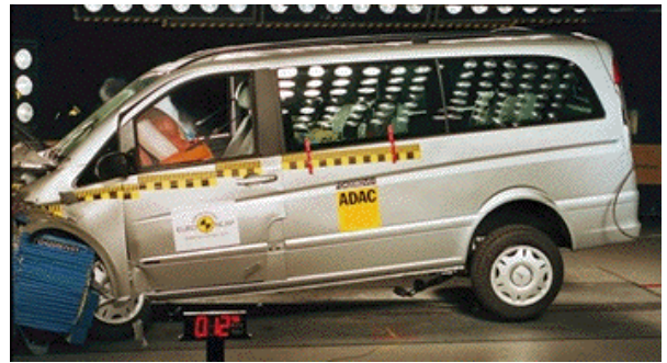
Offset crash test at 64km/h
