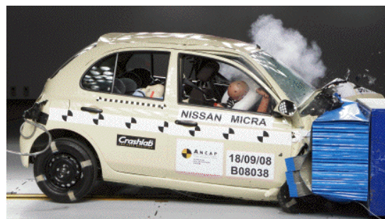
Offset crash test at 64km/h
