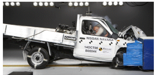
Offset crash test at 64km/h
