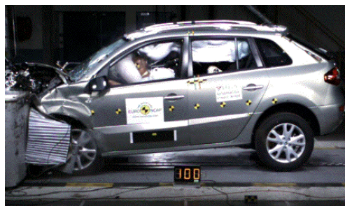
Offset crash test at 64km/h
