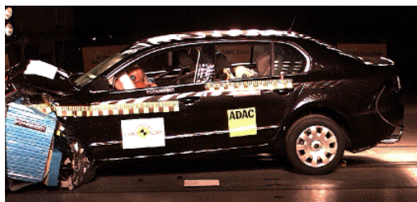
Offset crash test at 64km/h
