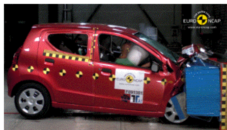
Offset crash test at 64km/h
