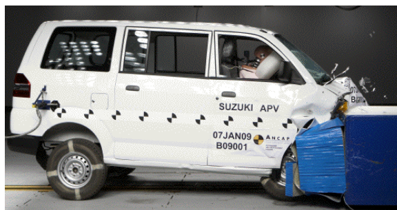
Offset crash test at 64km/h
